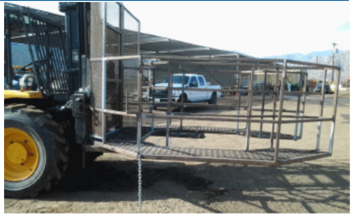
The platforms are mounted on lift trucks and can reach high into date trees for needed work.
